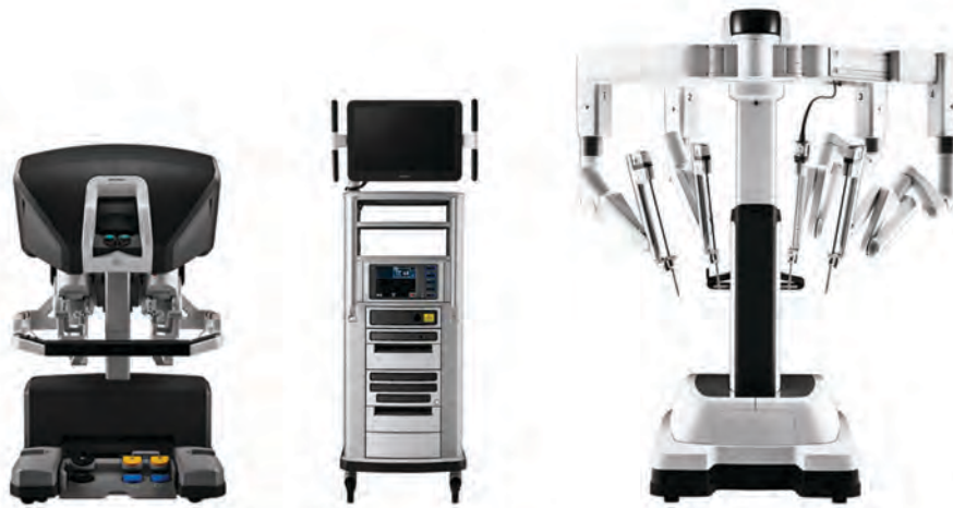
From left, the da Vinci Xi Surgical System surgeon console, vision cart and patient cart.
